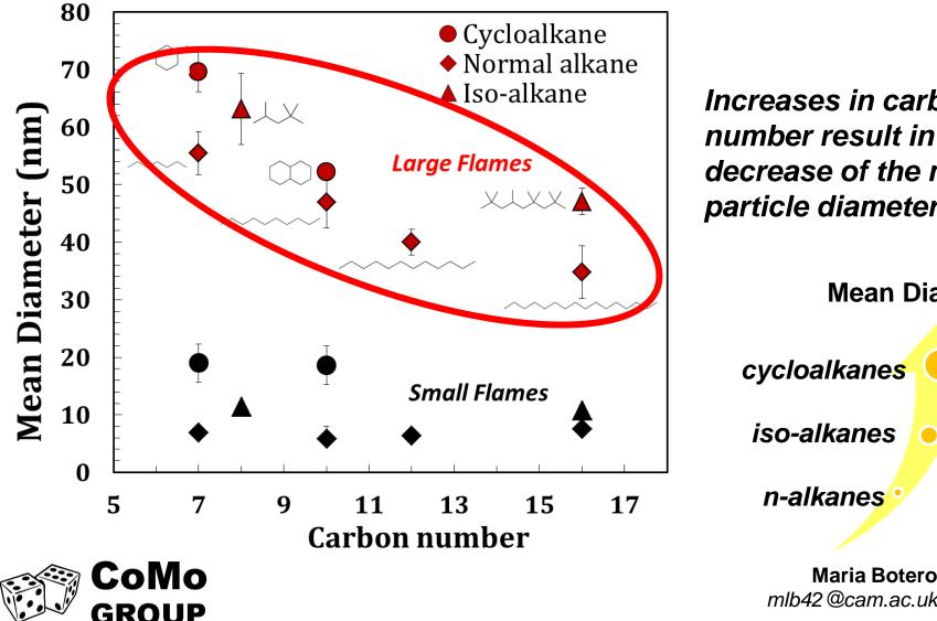
Increases in carbon number result in a decrease of the mean particle diameter
