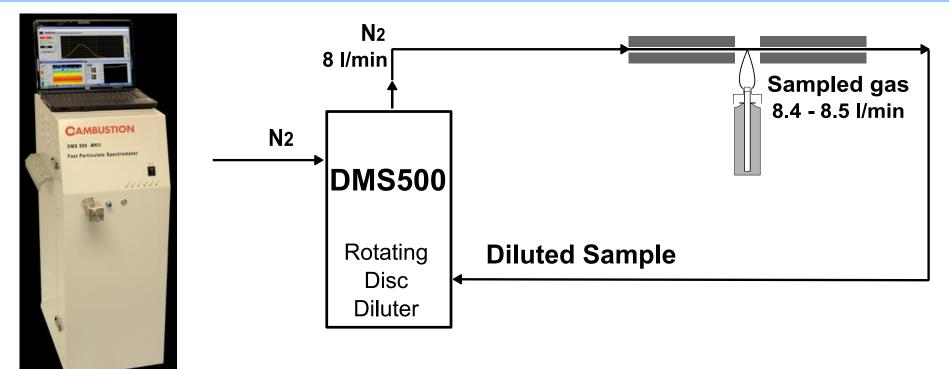
DMS500 is a fast particle analyzer that enables to measure PSD in real-time. Particles are sized based on their mobility diameter
